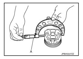
Piston-to-Cylinder Bore Clearance
