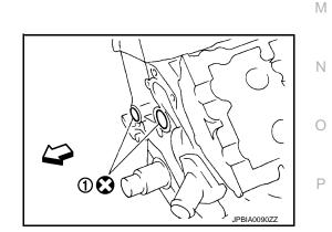
b. Apply liquid gasket with the tube presser (commercial service tool) to rear timing chain case back side as shown in the figure. Use Genuine RTV Silicone Sealant or equivalent. Refer to GI-22, "Recommended Chemical Prod-
