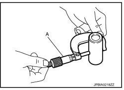
Piston to Piston Pin Oil Clearance
