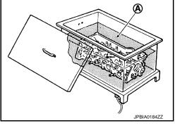
c. Provide valve seats (EXH) cooled well with dry ice. Force fit valve seat (EXH) into cylinder head. WARNING:
