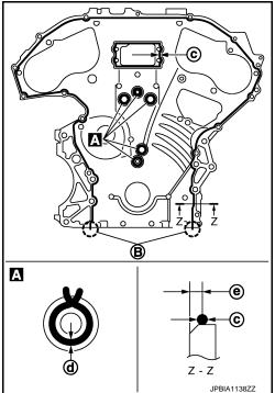
b. Apply liquid gasket to top surface of oil pan (upper) as shown in the figure.
