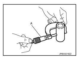
Connecting Rod Bushing Oil Clearance
