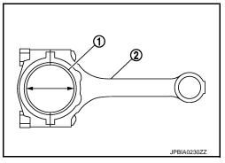
• Measure the inner diameter of connecting rod bearing with an inside micrometer.
