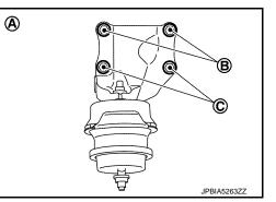
• Check that all engine mounting insulators are seated properly, then tighten mounting nuts.
