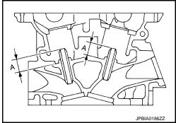
Using the valve guide drift (commercial service tool), press valve C. guide (EXH) from camshaft side to the dimensions as shown in the figure.
