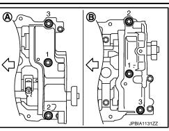
3. Remove front timing chain case, camshaft sprockets, and timing chain. Refer to EM-55, "Exploded View".
