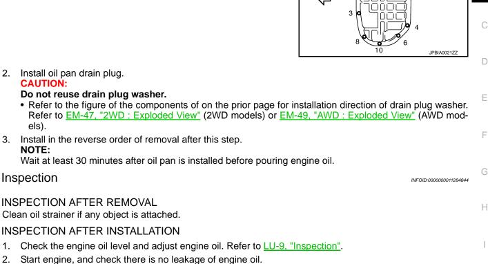
3. Stop engine and wait for 10 minutes. Check the engine oil level again. Refer to LU-9, "Inspection". 4.
