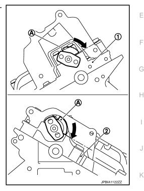
• If control shaft cannot be moved, set crankshaft in position referring to the information below. (To displace cam nose)
