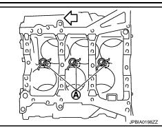
4. Install main bearings and thrust bearings as follows: CAUTION:
